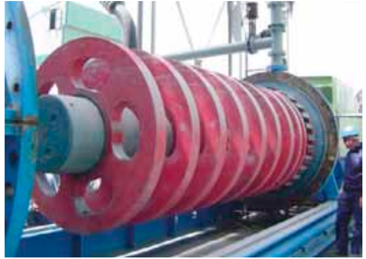
Internal view of grinding discs in M10,000 IsaMill™
