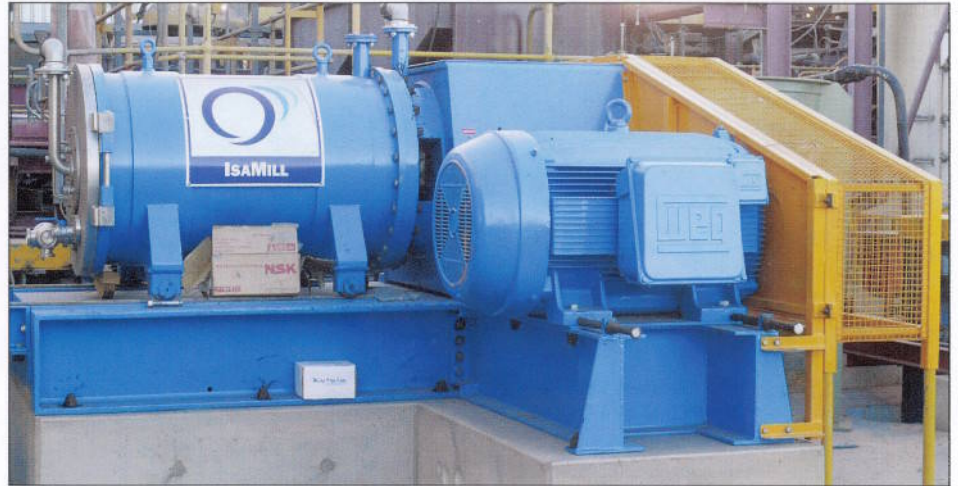
SMALL SCALE M500 ISAMILL TAKING UP AN AREA OF LESS THAN 10 SQUARE METRES IS IDEAL FOR RETROFITTING INTO EXISTING CONCENTRATORS, OR GREENFIELD OPERATIONS
