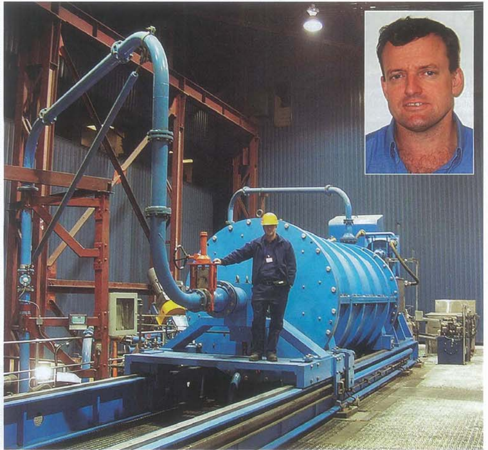
IsaMill manager – South African Projects Dan Curry atop a M10,000 IsaMill. Inset: Brenton Burford: "design the most efficient circuit possible from an energy perspective; don't grind unless you have to"
