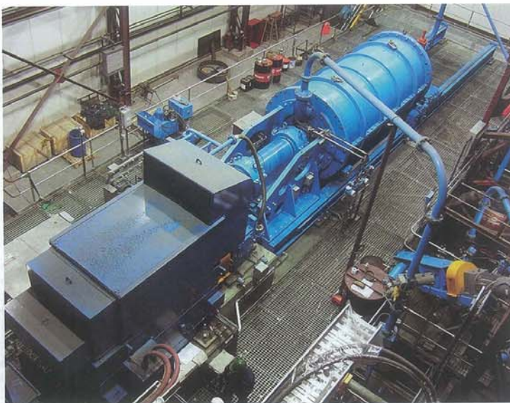
The M10,000 IsaMill at the Kumtor Operating Company, a subsidiary of Centerra Gold, in the Kyrgyzstan Republic
