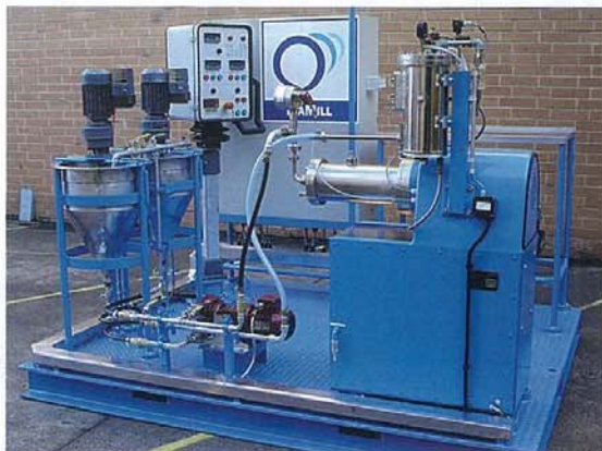
15 kg samples are required to be passed through the mill a number of times until the required grind size is achieved.
