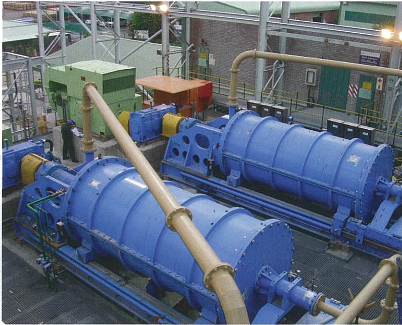
Two 10,000-litre volume IsaMills located at the Mogalakwena Mine in South Africa.
