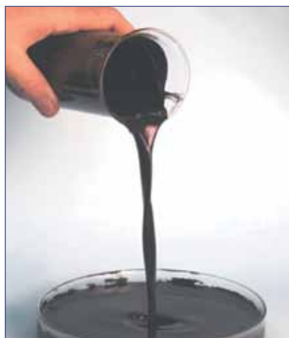
MRC containing 0.8% ash and with an SE of 19 MJ/L (gar)
