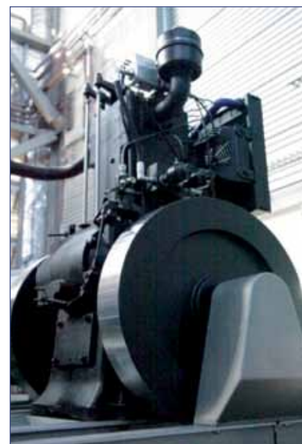
A 3.9L laboratory coal engine adapted with electronically controlled fuel injection
