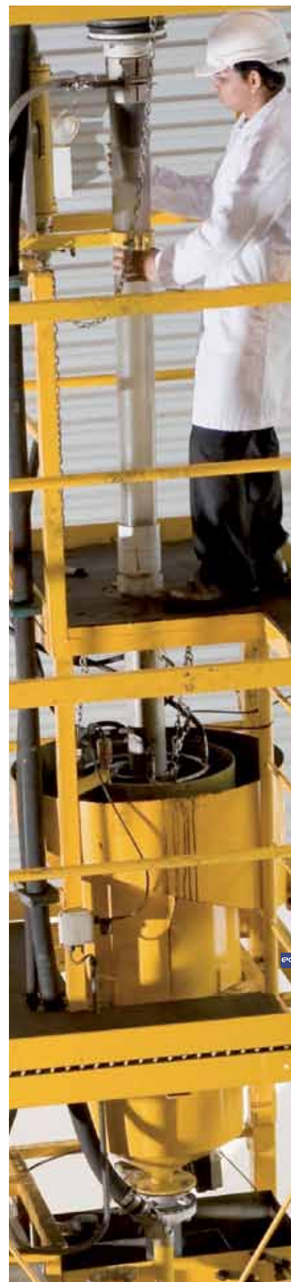
Producing MRC at CSIRO using an L500 J-cell courtesy of Xstrata Technology
