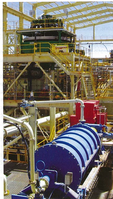
An Xstrata Jameson Cell and IsaMill in use at Prominent Hill in Australia.
