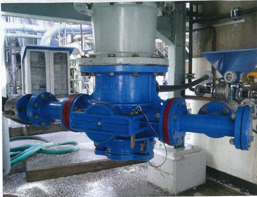
Xstrata Technology's new IsaCharger is a media addition system for IsaMills; it has no moving parts and uses water induction to transfer media to the mill.
