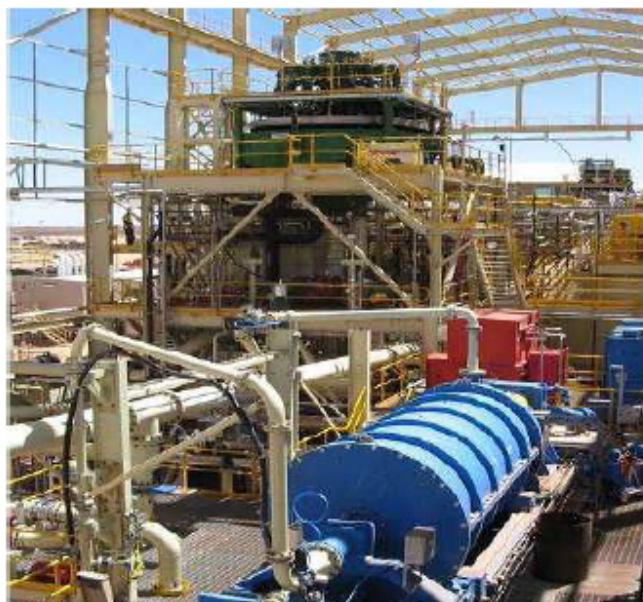
Exhibit 9: Prominent Hill Plant -IsaMill/Jameson Cell (LHS) and Banks of Flotation Cells (RHS)
