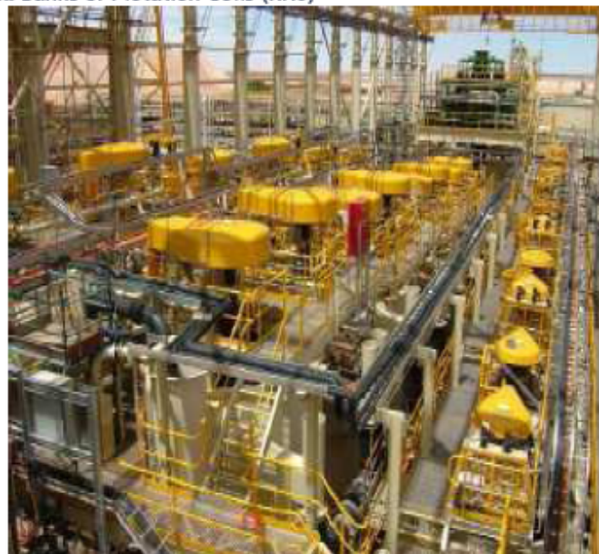
Exhibit 9: Prominent Hill Plant -IsaMill/Jameson Cell (LHS) and Banks of Flotation Cells (RHS)
