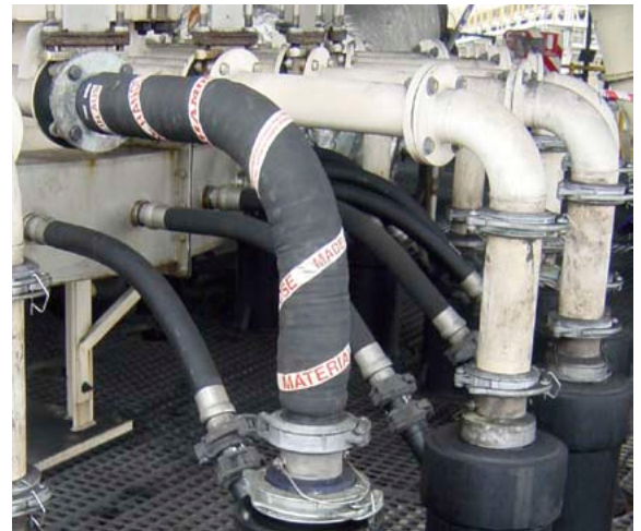
The Mark IV downcomer with simplified slurry feed piping against an older Mark III downcomer
