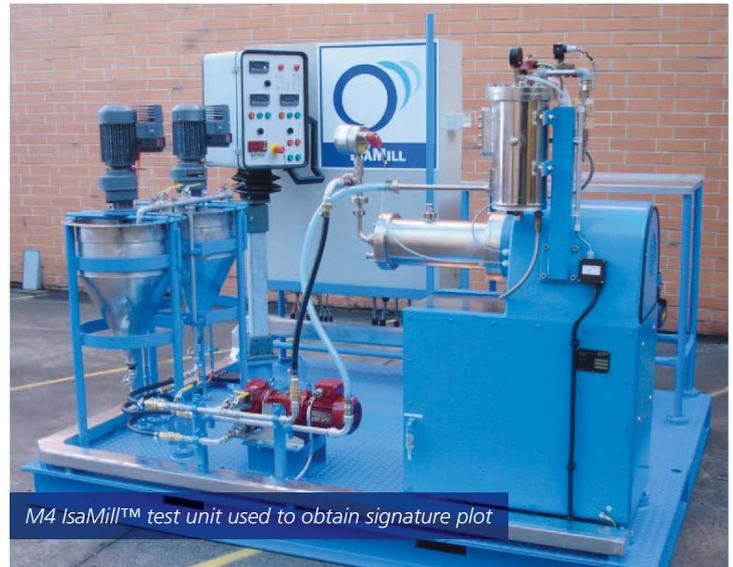
M4 IsaMill™ test unit used to obtain signature plot
